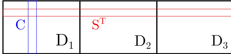
Figure A.4: Concatenation of three datasets, \mathbb{D}_1 , \mathbb{D}_2 and \mathbb{D}_3 . A matrix with the same number of rows of each dataset and number of columns equal to the sum of the number of columns of all datasets is obtained. The columns of the \mathbb{C} matrix (red) contains information relative to a single dataset, whereas the rows of the \mathbb{S}^T matrix (blue) necessarily contain information of all of them.
